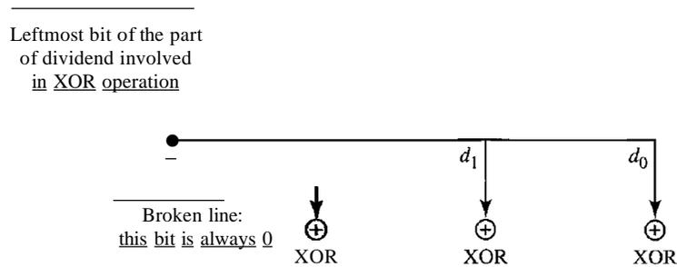
Note that if the leftmost bit of the part of dividend to be used in this step is 1, the divisor bits ( $d_2d_1d_0$ ) are all 1; if the leftmost bit is 0, the divisor bits are 000. The design provides the right choice based on the leftmost bit.
