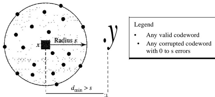
In Figure 10.8,  $d_{\min}$  must be an integer greater than  $s$ ; that is,  $d_{\min} = s + 1$ .
