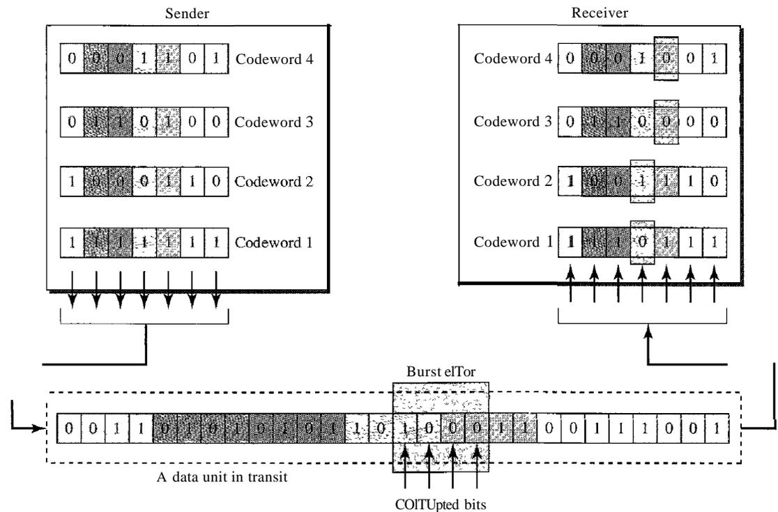
that when a burst error of size 4 corrupts the frame, only 1 bit from each codeword is corrupted. The corrupted bit in each codeword can then easily be corrected at the receiver.
